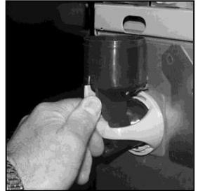
3. Pull off the impeller and the rubber seal.
