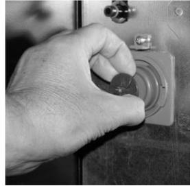
9. Line up the mixing system to the base unit ensuring that the green lever is turned to the left. Press the mixing system home on to the base unit and press and turn the green locking mechanism to the right to lock in place.
