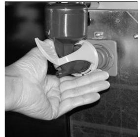
5. Remove the extract tray from the machine. Using a dry brush, clean the area under the extract tray.
