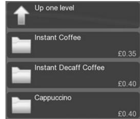
2. To change the price of the Instant Coffee, select **Instant Coffee**. The LCD will change and display the screen as shown below. To update the price, e.g. increase to 45p, press 4-5 using the appropriate touch-pads.
