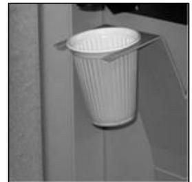
5. Refit the drip tray and cup catcher assemblies, ensuring that the drain tube from the cup catcher moulding is located correctly at the rear of the tray.
