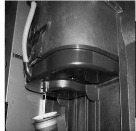
3. Clean the cup catcher and drain pipe in the sanitizer solution. Rinse the components with clean water and dry thoroughly. Wash the drip tray and grille thoroughly and sanitise using the diluted bactericidal cleaner solution.
