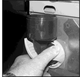
11. Press the securing tabs on each side of the dispense block and slide the block off the dispense head.
