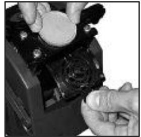
Take one cleaning tablet (supplied in packs of 30 - CMS part no. ZC10598000) and place it into the brewer chamber as shown.
