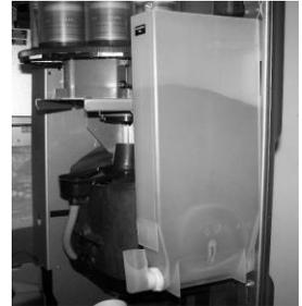
Place the canister into the canister filling station located on the door and fill canister with the correct ingredient.
