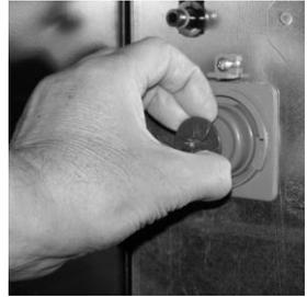
9. Line up the mixing system to the base unit ensuring that the green lever is turned to the left. Press the mixing system home on to the base unit and press and turn the green locking mechanism to the right to lock in place.
