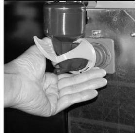
5. Remove the extract tray from the machine. Using a dry brush, clean the area under the extract tray.
